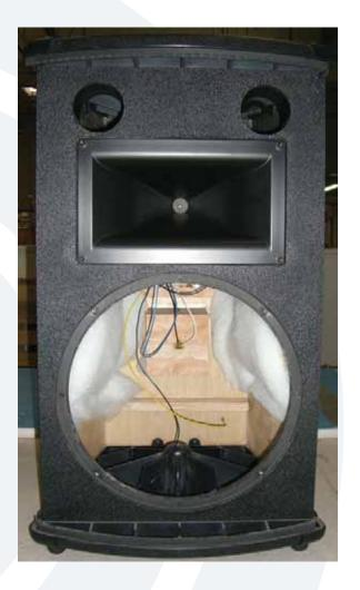
The picture above shows what the S215 looks like with the grill and woofer removed. Place the new woofer (part #0010658) where the old one was. Follow the same steps as above, but backwards 6 to 1. Power up the S215 and the new woofer should now be pumping out glorious lows. Awesome, you just replaced a 15" woofer!
